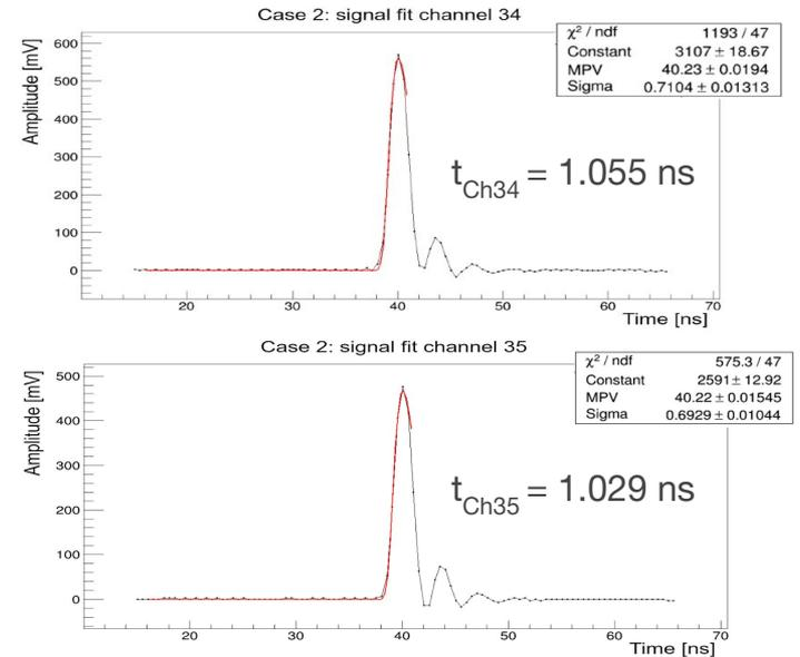
The rise time of *Ch35* is larger when it alone receives the most signal relative to the case when the signal is almost equally shared between *Ch34* and *Ch35*.
