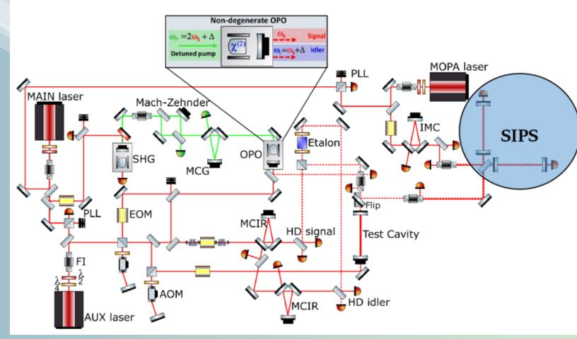
In the proposed design, the EPR signal field matches the interferometer's laser frequency, making it resonant in the Fabry-Perot arm cavities. Meanwhile, the EPR idler beam is slightly detuned, treating the interferometer as a filter cavity that rotates the squeezing ellipse.
