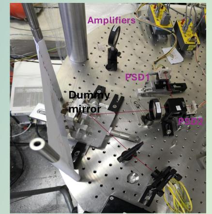
To optimize the alignment of the beam to ensure proper focusing on the image plane and minimize aberrations.
