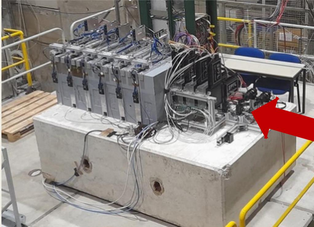
In August 2023, the detector was exposed to hadron beams with energies ranging from 100 to 300 GeV with known direction.
