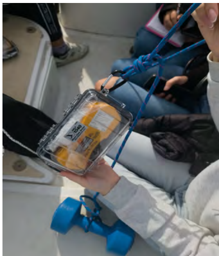
Geiger counter inside the waterproof container
