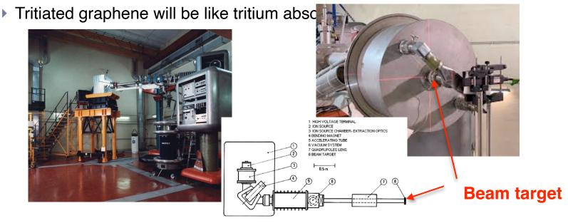
The whole vacuum chamber of the FNG is connected to a tritium detection system Beam target kept in a glove box Exhaust sent to atmosphere
