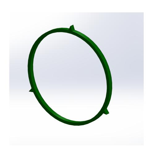
Geometry already tested in the XENON cryogenic pipe. Construction material will be Torlon.
