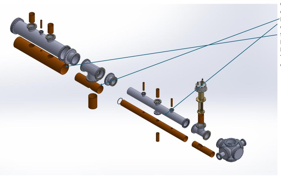
Copper shield to keep the filter environment in cold (protected by radiation). Probably the copper will be Gold plated and for sure a superinsulation blanket will be installed between copper and outer shell. The copper shield will be equipped with T sensors.
