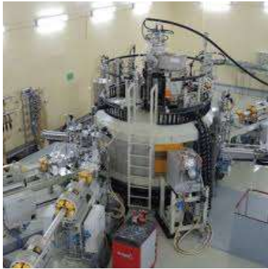
IBA Cyclone 30 30 MeV, 800/1500 \mu\text{A}
