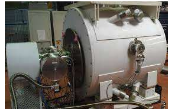
PMB-ALCEN Isotrace 12 MeV, 100 \mu A
