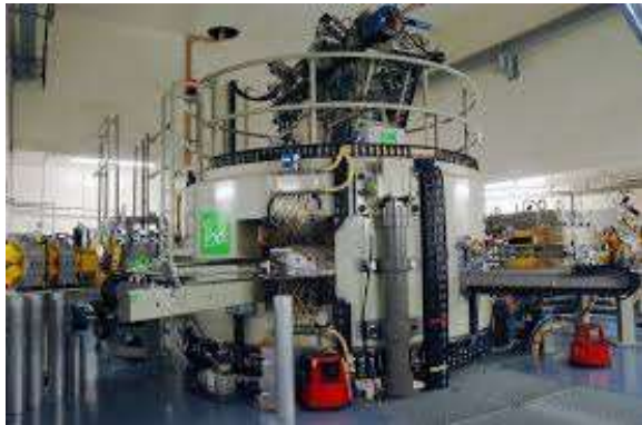
IBA Cyclone 70 30-70 MeV, 750 \mu\text{A}
