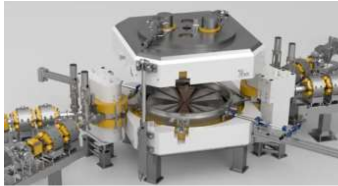
IBA Cyclone IKON 13-30 MeV, 500..1500 \mu\text{A}
