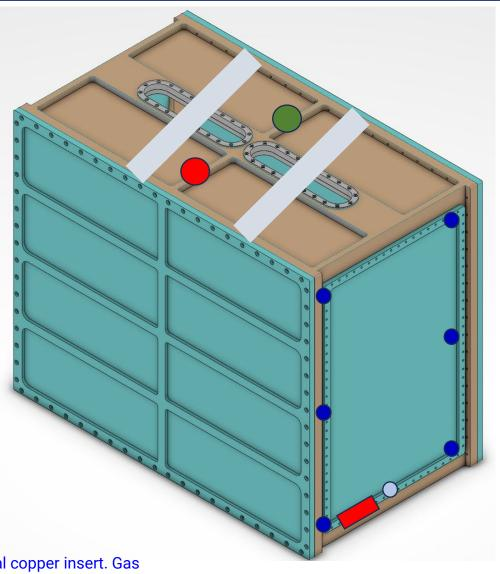
PMMA with cylindrical copper insert. Gas tightness ensured by PMMA filling in the cylinder hole
