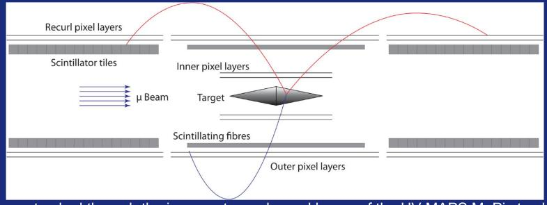
Electrons and positrons are tracked through the inner, outer and recurl layers of the HV-MAPS MuPix tracker Ultra low mass tracker with  $\sim 0.1\% X_0$  per layer. (50-70 µm sensors, low mass supports, cooled with gaseous Helium)
