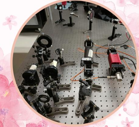
My PhD focuses on adaptive optics, specifically on studying wavefront deformations in the Extremely Large Telescope (ELT). My project involves the design of the "CiaoCiao WFS," a rotational shearing interferometer proposed as part of the MORFEO project, which aims to sense discontinuities in the ELT's segmented pupil. This work includes the implementation of the system at the Arcetri Laboratory and the development of software for data analysis.
