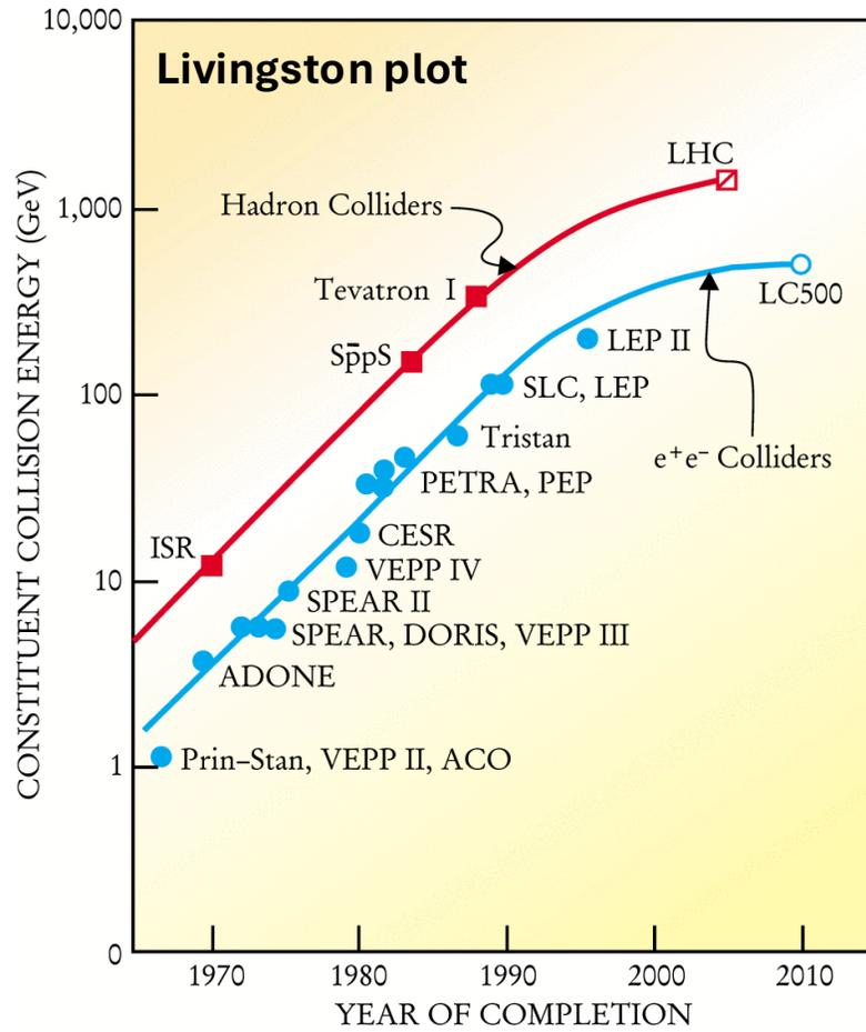
E+ e- circular colliders play a very important role in the development of HEP: up to the '80s they are discovery machines (**tau** lepton, **charm** and **beauty** quarks). At higher energies (= mass of particles to be discovered) the synchrotron radiation limits the energies reachable.
