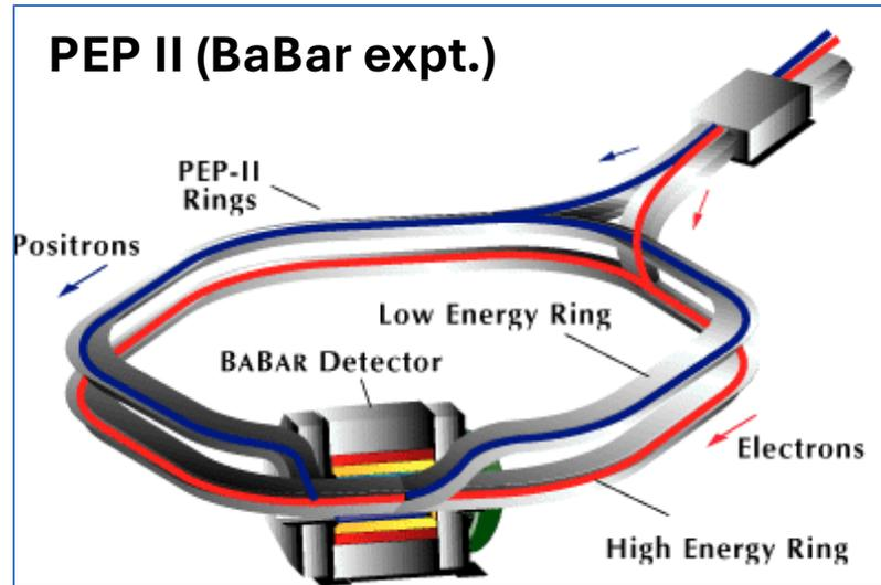
High luminosity  $e^+ e^-$  circular colliders **PEP II** (SLAC), **KEKB** (Tsukuba), **DAFNE** (Frascati), built to study the problem of asymmetry in the Universe between matter and anti-matter in different initial states: **B mesons** (PEP II, KEKB) and **K meson** (DAFNE). KEKB still active.
