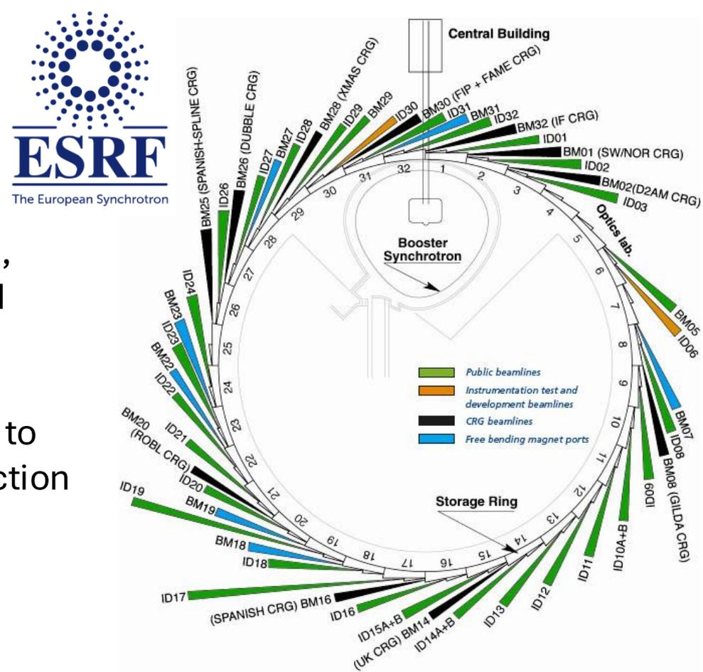
ESRF (Grenoble) is among the most advanced machines which recently underwent an upgrade from 3<sup>rd</sup> generation to 4<sup>th</sup> generation SM to increase the brilliance (= intensity) of photon beamlines, following the developments **studied for future Flavor Factories (Hybrid Multi Band Achromat)**, where dimension of e- beams which are at the limit of theoretical diffraction of the emitted radiation
