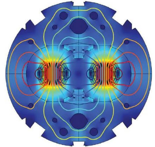
Magnetic Resonance Imaging scanners make large use of SC cables to achieve the very high field needed (3 T commercial, with R&D up to  $\sim 10$  T). Nb<sub>3</sub>Sn and HTS cables (**ReBCO**) are used for fusion toroids (e.g. ITER) to confine with high magnetic field the plasma
