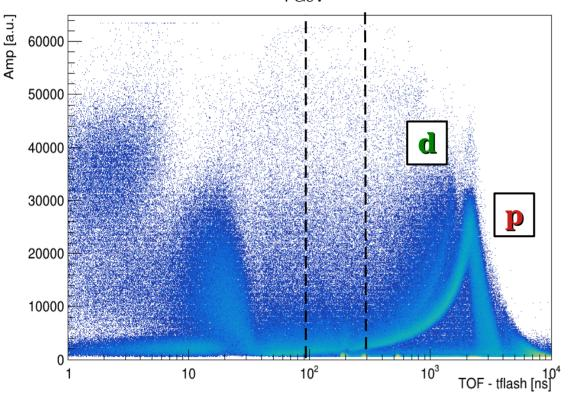
protons punch-through at neutron Energy ~ 20 MeV
