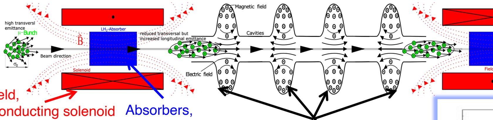
High-field, superconducting solenoid to minimize multiple scattering effect
