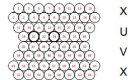
Prototype 2: 10 mm tube area only. Two planes of X, two planes of U (2'), two planes of V (-2') and two planes of X.
