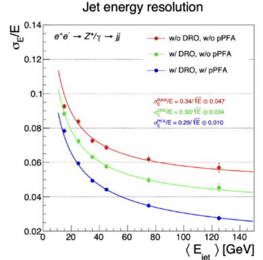
Particle flow + hybrid segmented calorimetry
