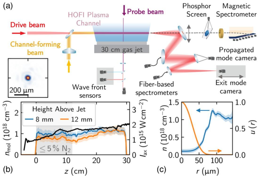
FIG. 1. (a) Schematic of the experimental setup. Inset: measured vacuum mode of the drive laser pulse. (b) Measured molecular density of the gas jet (blue and orange lines) and peak intensity of the channel-forming pulse along the length of the gas (black line). (c) Measured electron and neutral density  $n = n_e + n_n$  of the HOFI plasma channel at  $\Delta\tau = 6$  ns (blue) and calculated fundamental mode of the measured plasma channel (orange line).
