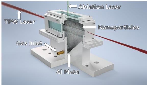
**FIG. 2.** A drawing of the gas cell. A 532-nm laser is focused through the top window onto the surface of a metal plate and generates the nanoparticles through laser ablation. The nanoparticles mix with the helium gas and fill the volume of the gas cell uniformly. The Texas Petawatt Laser enters the gas cell through a 3-mm-diameter pinhole and generates electrons that exit the gas cell through another 3-mm pinhole.
