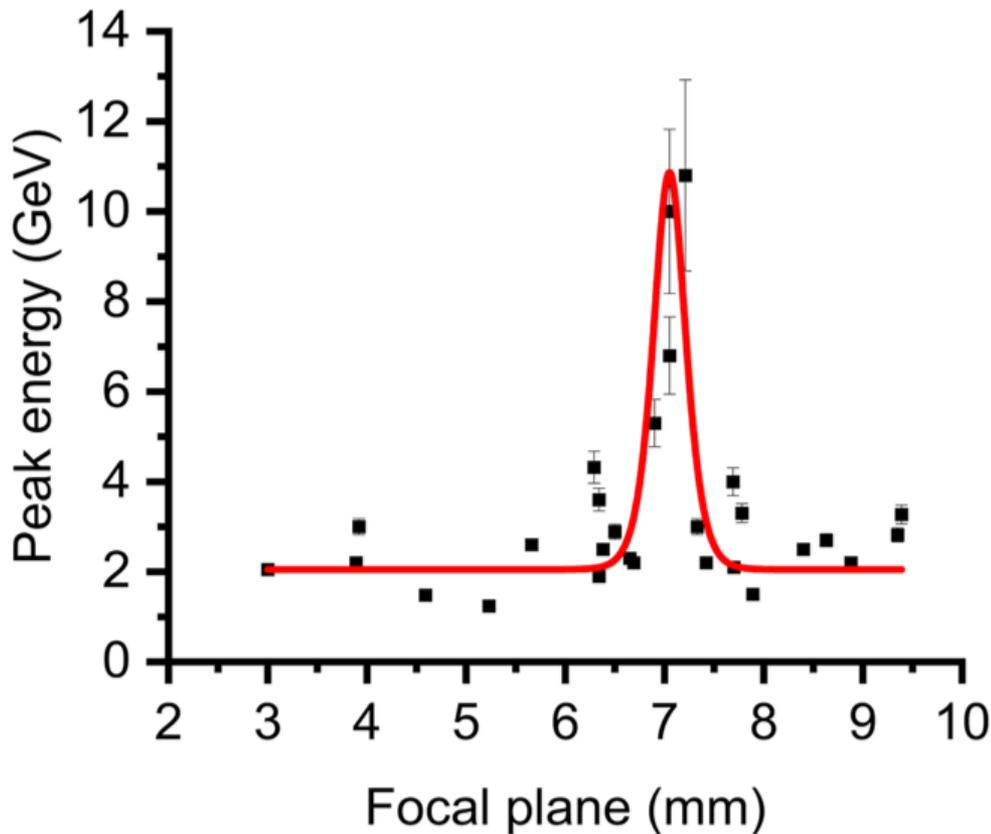
**FIG. 11.** The dependence of the maximum (or cut-off) electron energy on the position of the laser focal plane in the gas cell. It can be observed that all the shots with electron energies above 3.5 GeV are grouped around  $7 \pm 1$  mm. The red curve is drawn to guide the eye, and the entrance pinhole is at 0 mm where the laser with a vacuum Rayleigh length of  $\sim 1.5$  cm is focused.
