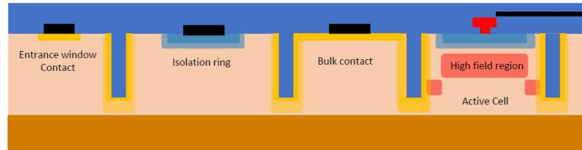
**D split** - border cell and isolation ring biased together unbiased trench
