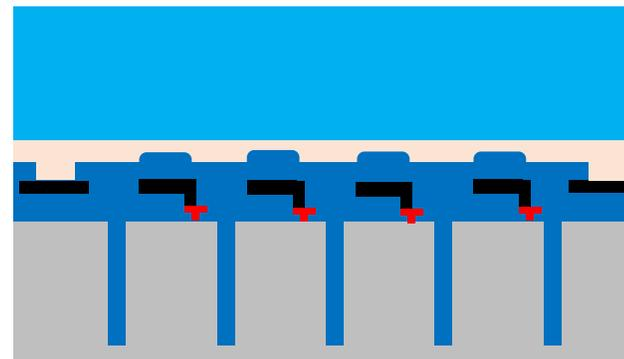
Doping Selective WET etching is used to complete the substrate removal and to reach the epi/sub interface by reducing the final TTV
