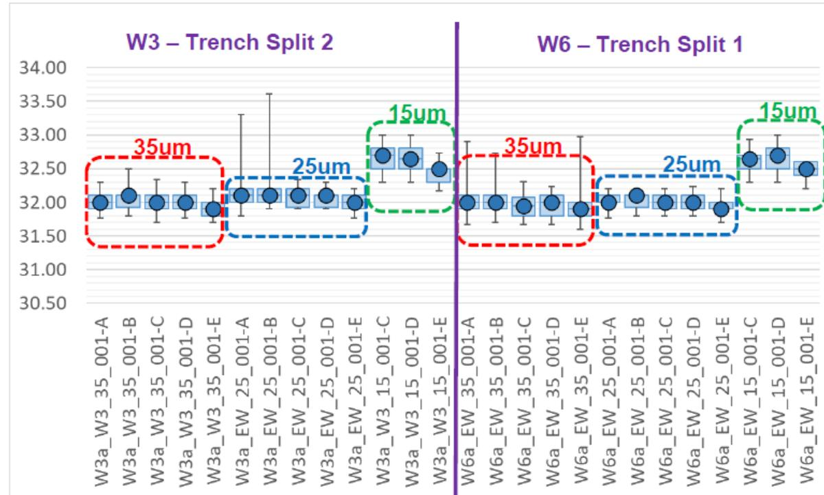
Quite uniform breakdown voltage between same splits and different wafers
