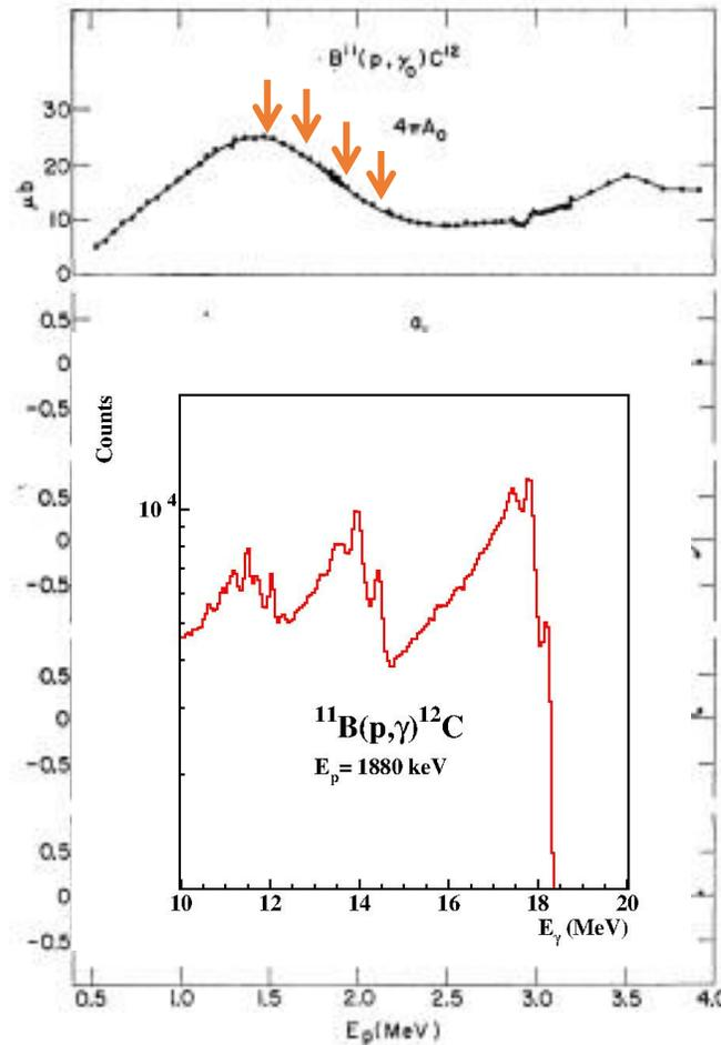
$\gamma$ -ray spectrum taken with a 3"×3" LaBr<sub>3</sub> detector.
