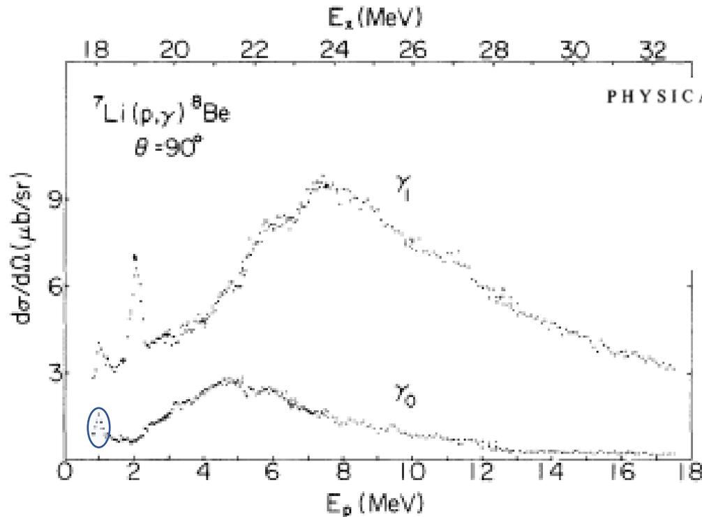
FIG. 3. The yield functions for the  $\gamma_0$  and  $\gamma_1$  transitions obtained at  $90^\circ$ , which show the broad giant resonances built on the ground state and the first excited state of  ${}^8\text{Be}$ .
