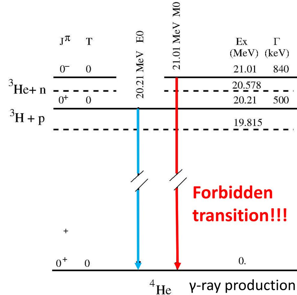
$\gamma$ -ray production with direct proton capture.
