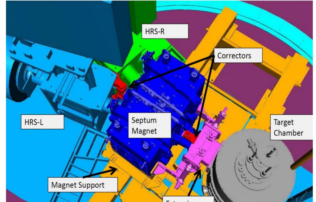
Electrons are detected in HRS-L while positrons in HRS-R
