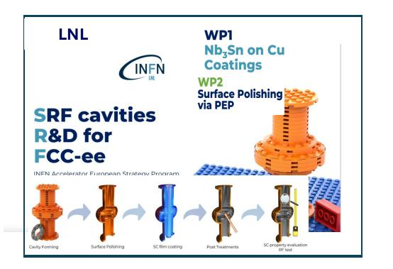
This solution can be used at higher temperatures than Niobium (4.5 K vs 2.0 K), with consequent important savings on the energy spent by the cryogenic system
