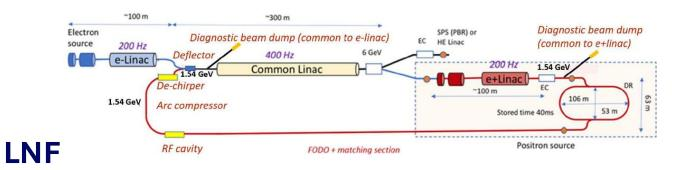
Necessary to "compress" the positron beam originating from the source until it reaches the characteristics necessary to carry out high-frequency collisions with the electron beam in the FCC-ee ring
