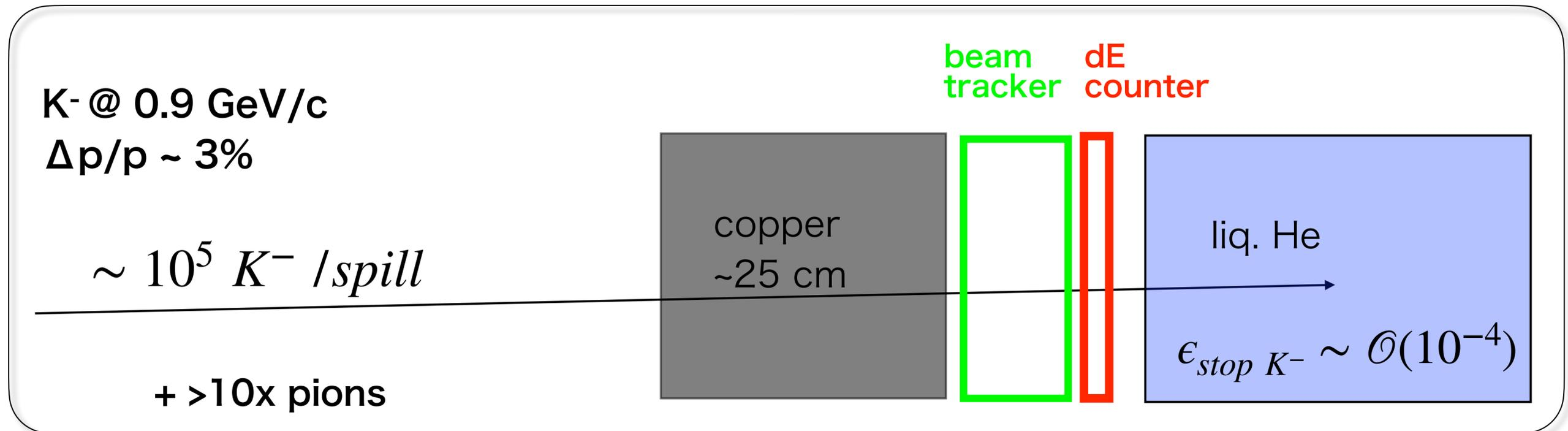
J-PARC provides higher intensity  $K^-$  — advantage with liquid target.
