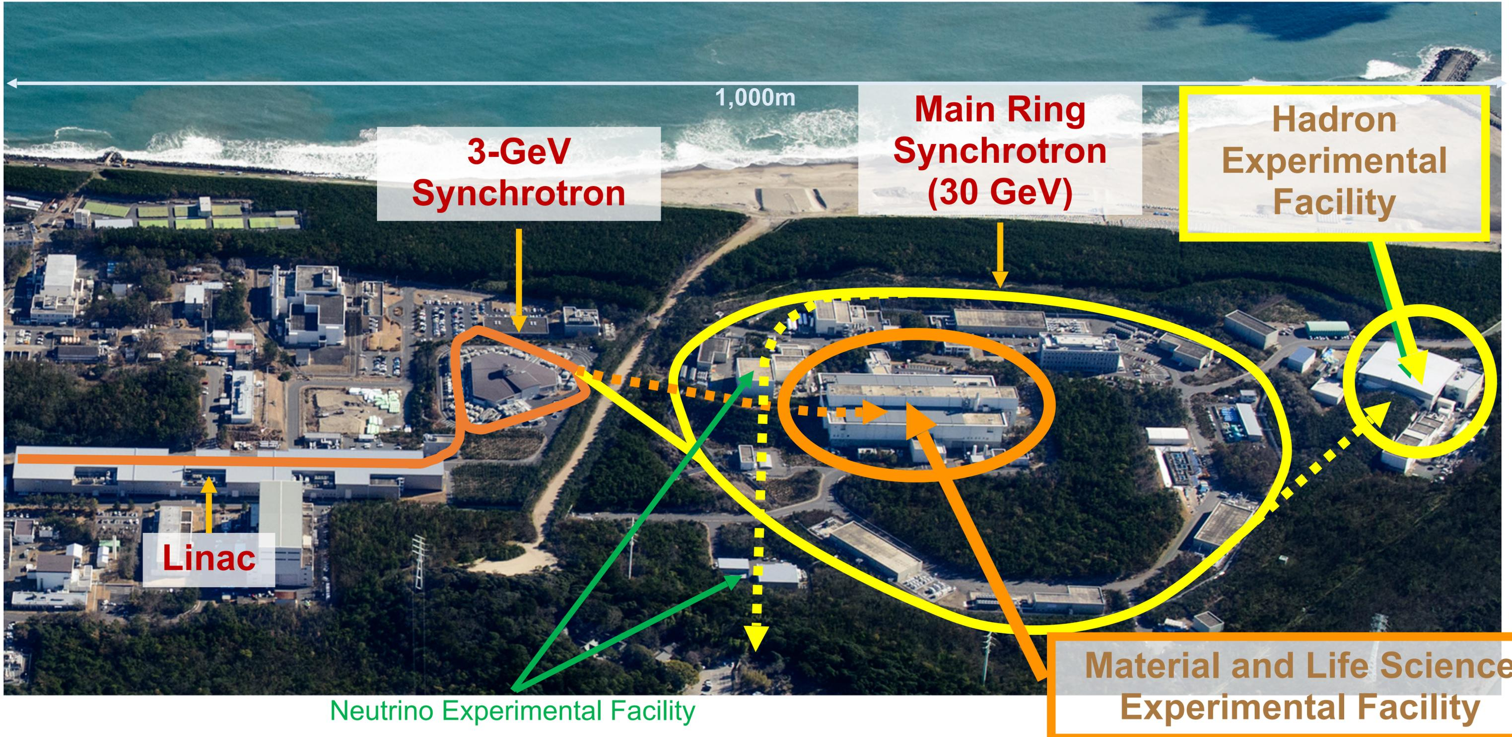
World's highest intensity proton driver → high-intensity secondary K/ $\mu$  beam
