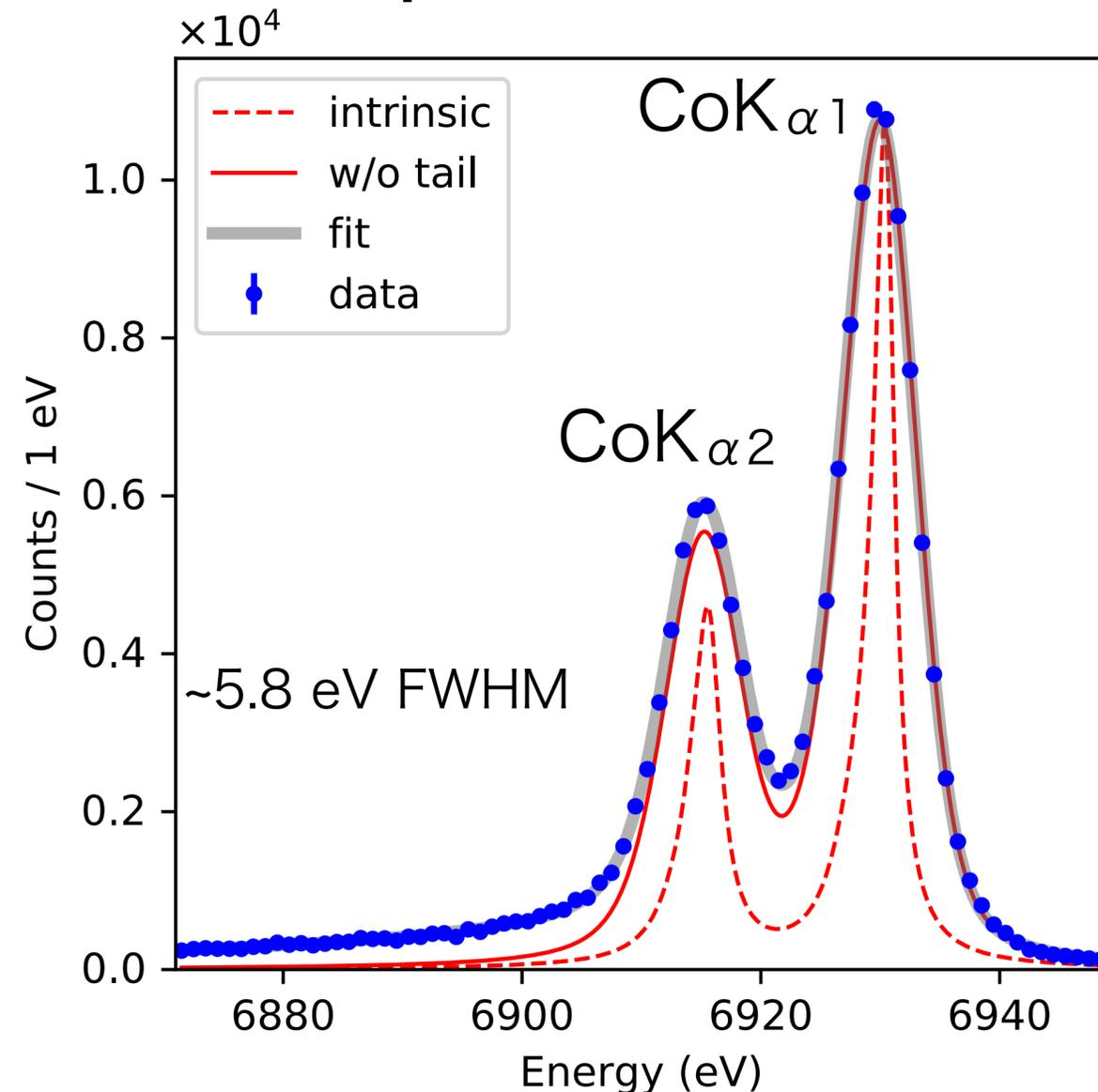
Detector response is well described by a gaussian and a low-energy exponential tail
