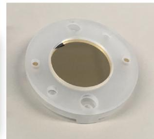
5  $\mu\text{g}$  vapor deposited Au
