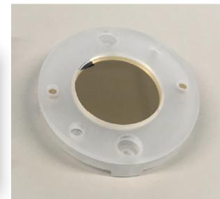
5  $\mu\text{g}$  vapor deposited Au
