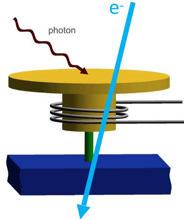
Michel electrons shoot through absorbers into silicon substrate and heat-up pixels “from the backside”
