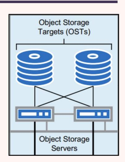
• when a server fails the remaining one becomes in charge of all resources (there might be a performance) loss but the system stays active), after making sure that the malfunctioning server will not come back alive
