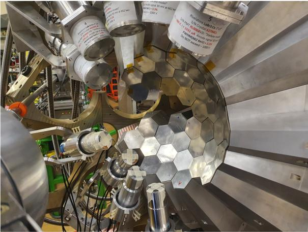
Fig. 1. The AGATA array with the absorbers installed at LNL.
