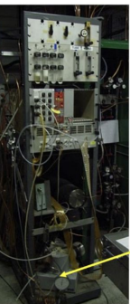
Deuterium UV lamp, Monochromator system, 1.6 m column for gas transparency measurement
