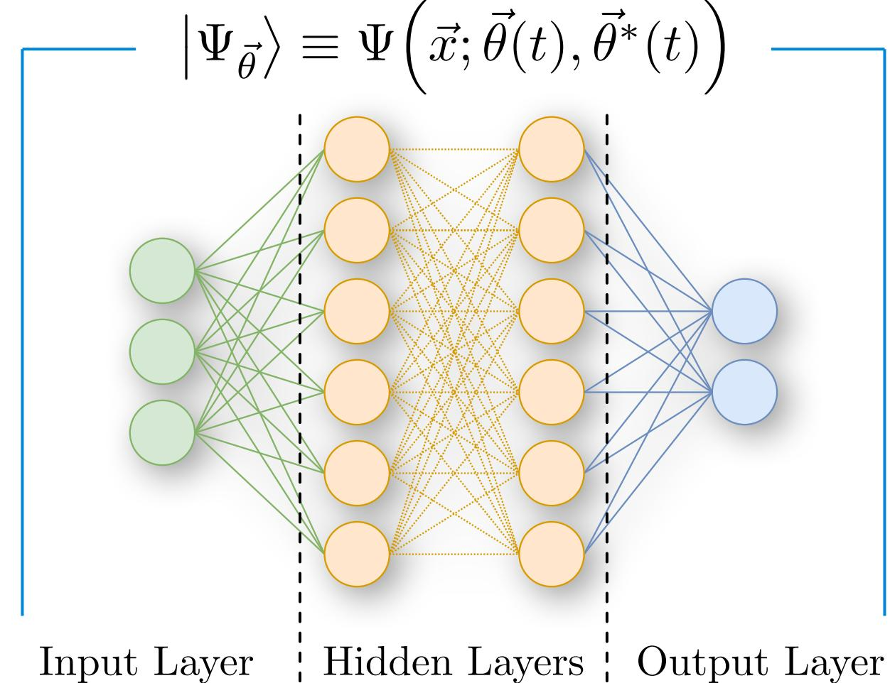
A NQS is a wavefunction ansatz parametrized by the weights and biases of an artificial neural network (NN).
