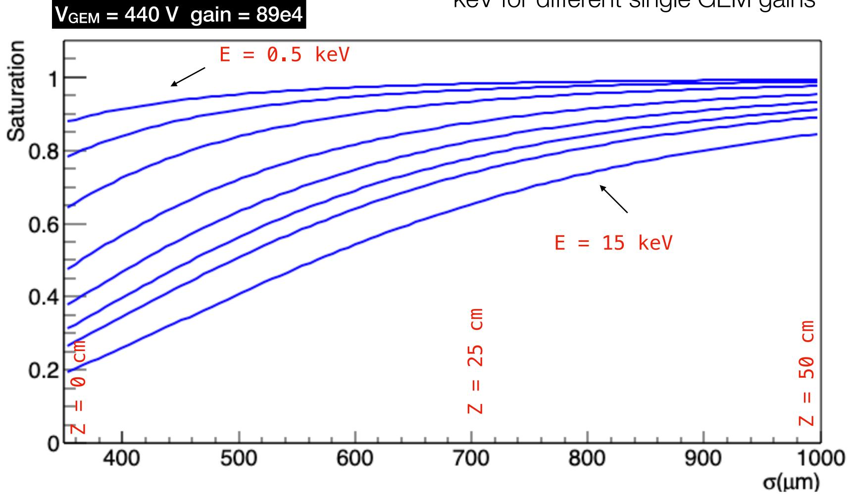
By using the fitted function and the fit results, one can evaluate the saturation as a function of energy released: 15, 10, 8, 6, 4, 2, 1, 0.5 keV for different single GEM gains
