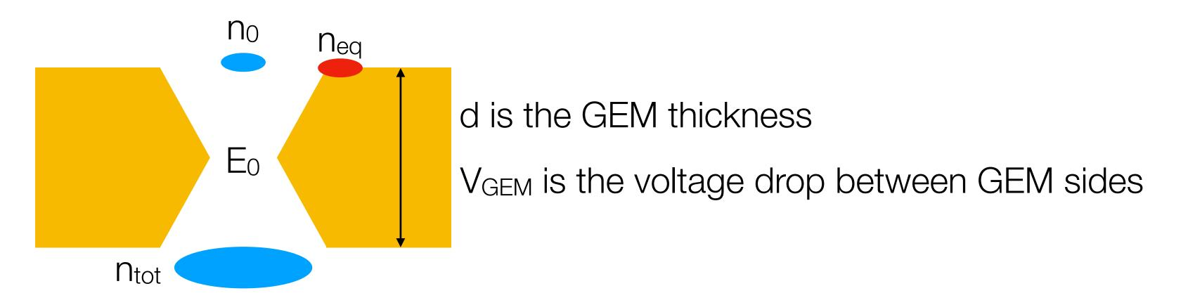
In fact we know that for  $V_{GEM} \ll V_{thr}$ , avalanches do not happen and the model doesn't work We can then write the not-saturated gain as
