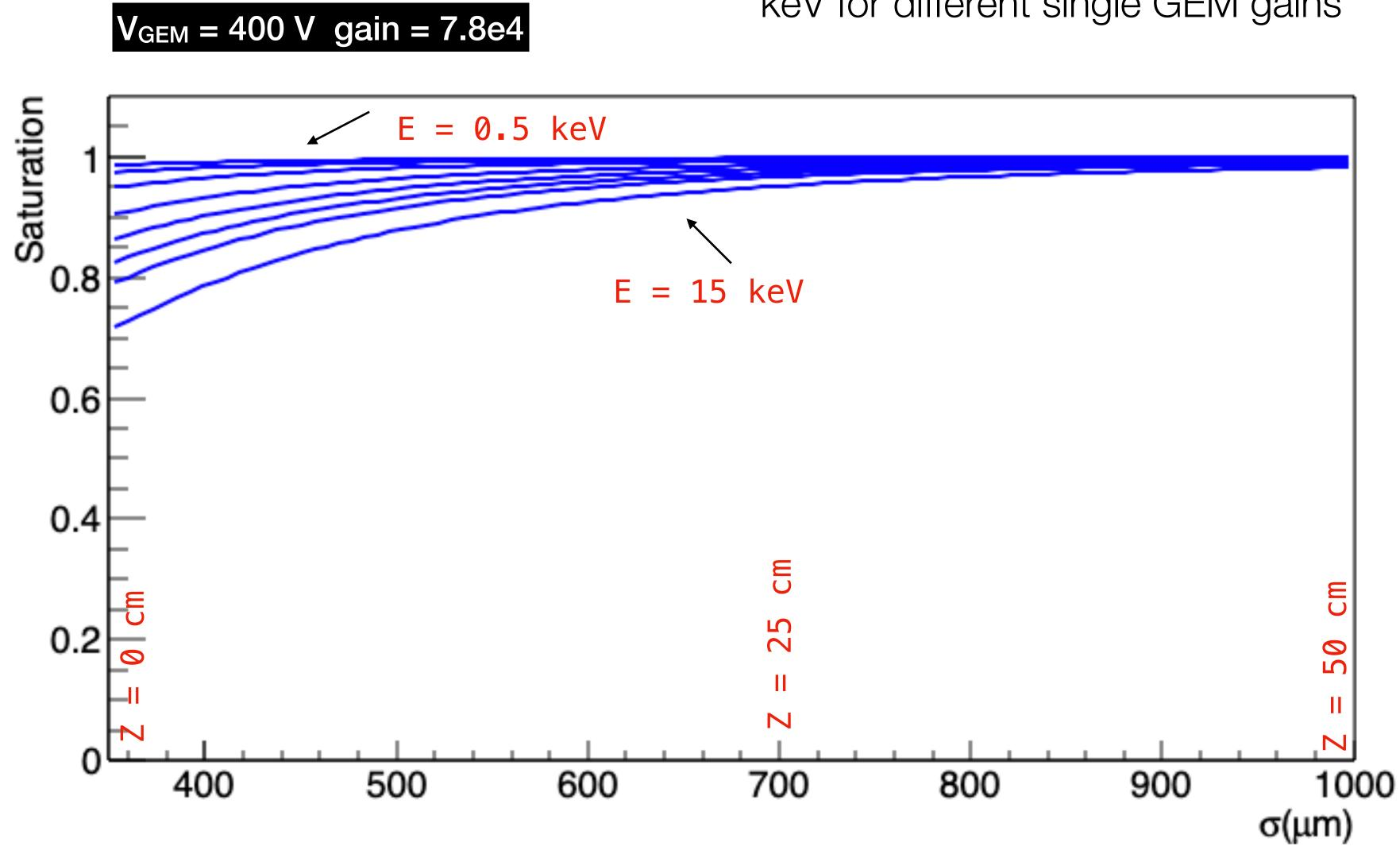
By using the fitted function and the fit results, one can evaluate the saturation as a function of energy released: 15, 10, 8, 6, 4, 2, 1, 0.5 keV for different single GEM gains
