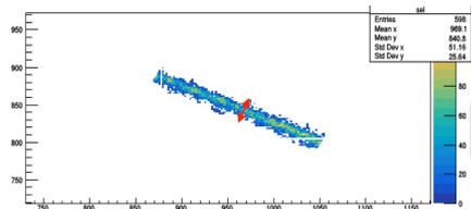
for production points farther in  $Z$  from the GEMs. This is reflected in the transverse ( $Y$ ) light distribution of each segment of the track: the  $\sigma_Y$  obtained from the Gaussian fit is in fact increasing with  $\sqrt{Z}$ . Therefore, the segment's original  $Z$  can be deduced by measuring  $\sigma$  (Fig. 8).
