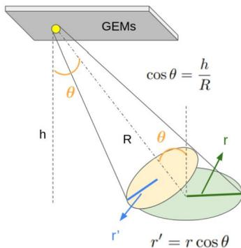
$$L_{PMT} = \frac{L_{spot}}{4\pi R_i^2} \frac{\pi r^2 h}{R_i}$$
