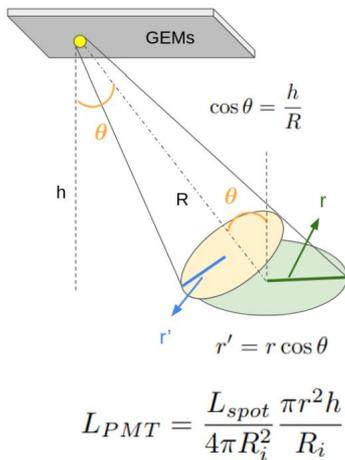
2. We apply a **multi-variable Bayesian fit** in a time window by **integrating the charge** ⇒ We retrieve **(x, y, L) information**
