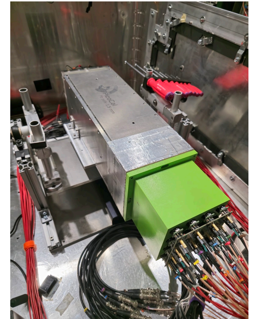
Picture of a Pb-polystyrene prototype in a test-beam setup
