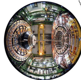
Open CMS detector, showing the endcap calorimeter sticking out, which will be replaced with the new high granularity calorimeter (HGAL) around 2024-2026.
