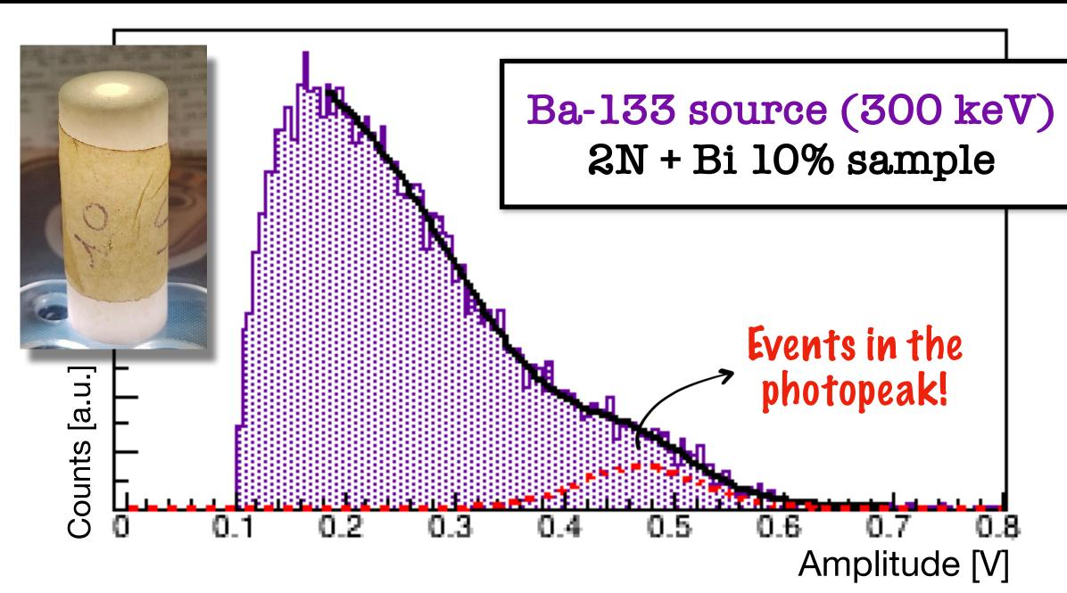
The addition of Bismuth does not deteriorate the time resolution!
