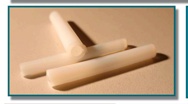
In order to improve the collection efficiency of the scintillation light, we produced samples where the polymerization process happens directly inside a PTFE (teflon) coating.
