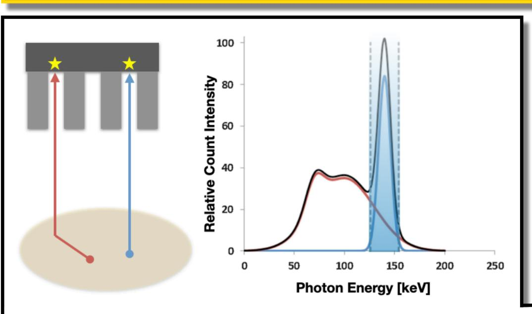
To reduce the discharge of "good" events, the probability of photoelectric absorption inside the scintillator must be maximized. Typically, inorganic scintillators are exploited due to their high atomic number.
