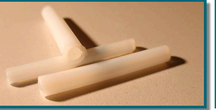
In order to improve the collection efficiency of the scintillation light, we produced samples where the polymerization process happens directly inside a PTFE (teflon) coating.
