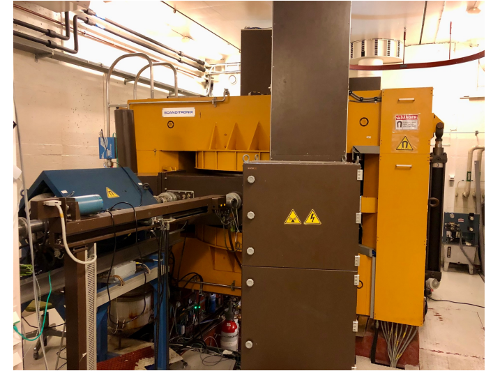
MC-35 cyclotron (p, d, ^3\text{He} , ^4\text{He} )
