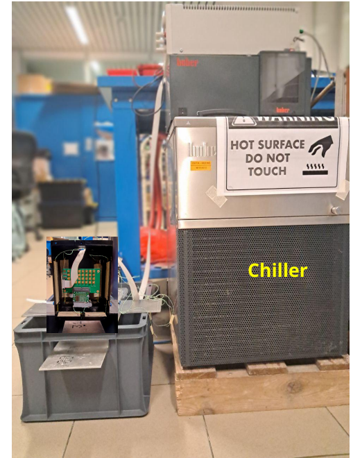
Chiller was used to regulate the temperature by continuous flowing of liquid
