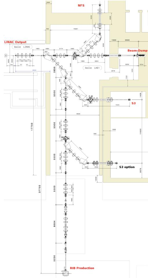
Figure 2: Detailed HEBT lines of SPIRAL2
