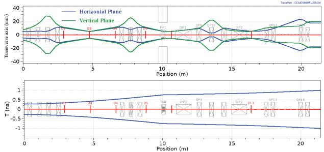
Figure 7: Transverses and longitudinal beam envelops at  $\pm 5\text{RMS}$  for Deuterons beam at 40MeV, 5mA from LINAC exit up to NFS area.
