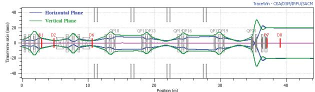
Figure 5: Transverses beam envelops at  $\pm 3\text{RMS}$  for Deuterons beam at 40MeV, 5mA from LINAC exit up to RIB production target
