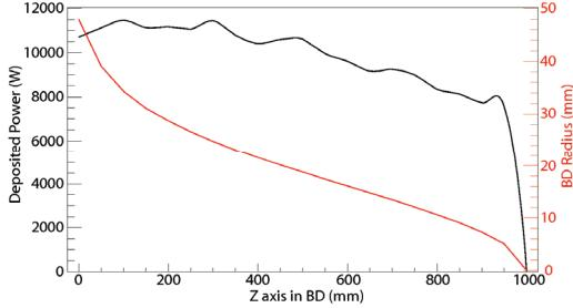
Figure 6: Beam-dump profil and deposited power for initial 200kW beam power
