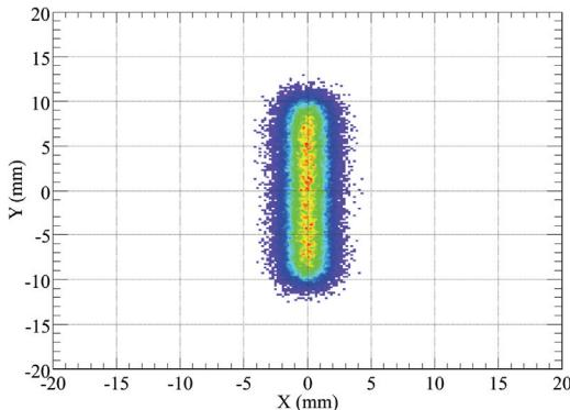
Figure 8: Integrated beam spot at the S3 target position for Heavy Ions with  $A/q=3$  to all energies.
