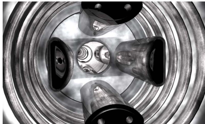
High Voltage Column (~Ø 6 inch) with ESQ Electrodes
