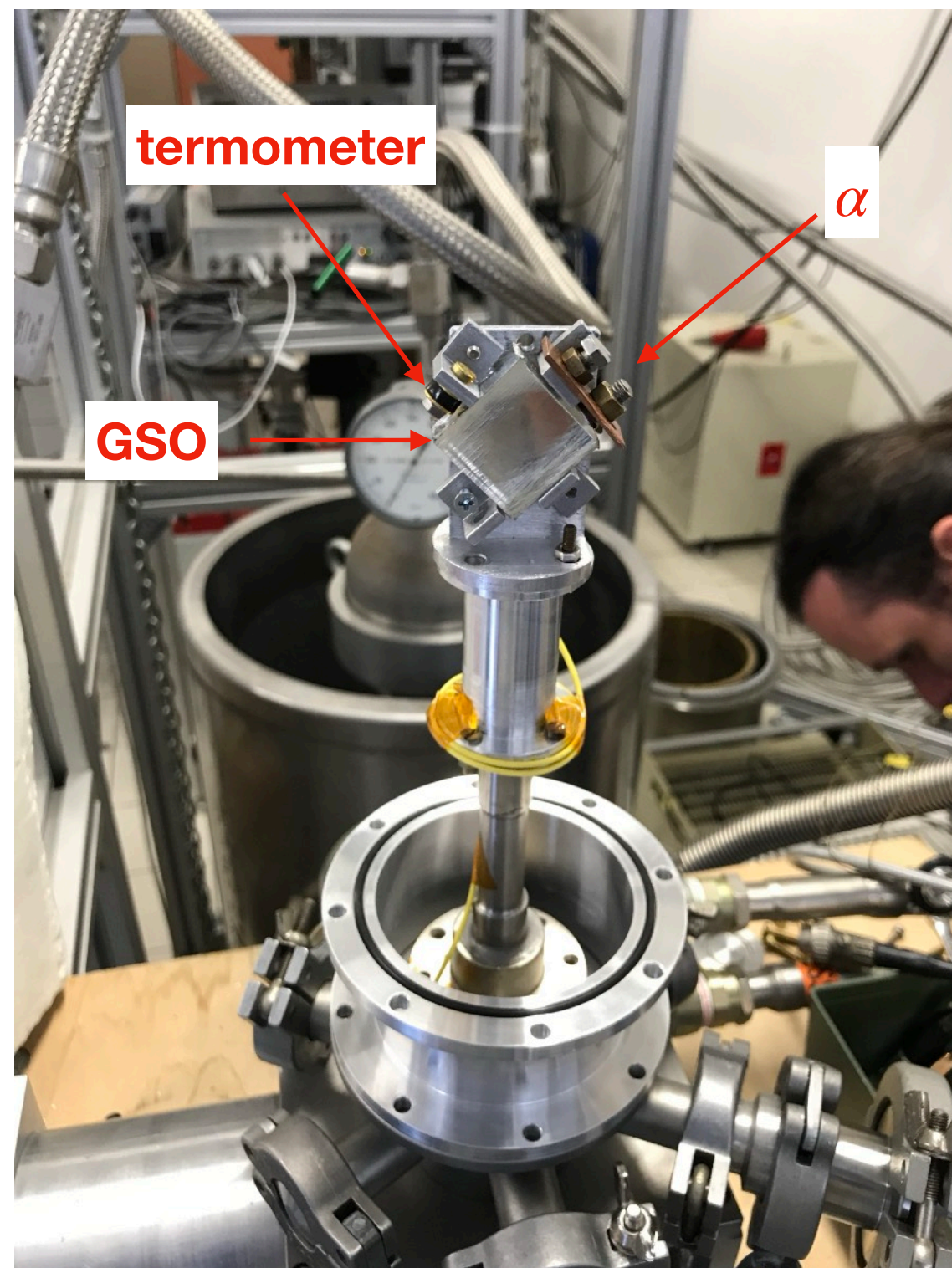
(Picture of preliminary tests. Actually the Crystal and the PMT have been moved to use the top window which allows a better light collection)
