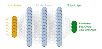
Input: W [1..6] - average wire position of the segment Output: track momentum and angles
