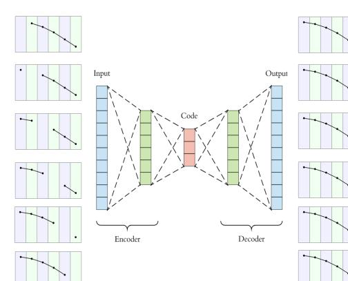
Good, 6-superlayers, reconstructed tracks are used to generate training samples by removing one of the segments
