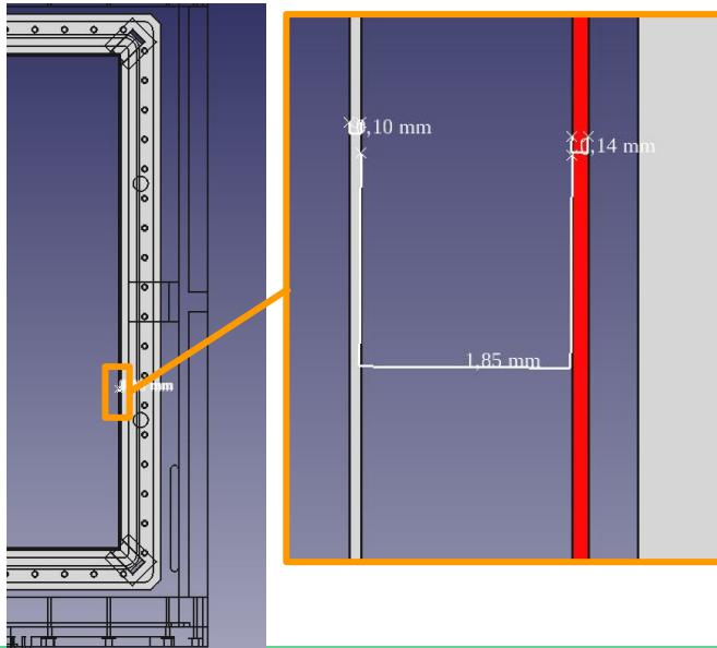
Implemented in CAD as a plastic layer of 100 um + 140 um thick Cu coils with a gap of 1.85 mm → ?
