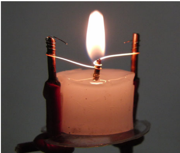
Fig. 6 A candle with a metallic artificial wick heated using an electric current
