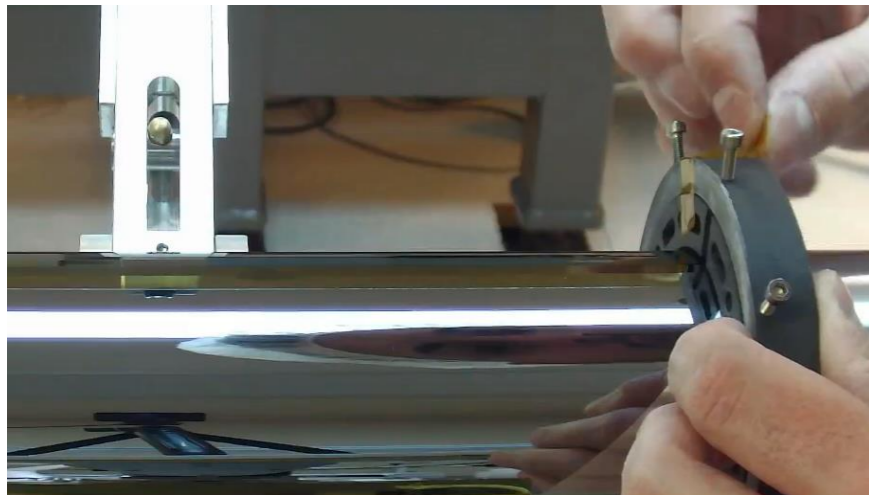
A. 1st half-ring + alignment tool
