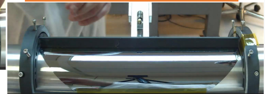
Insertion of 2nd alignment tool
