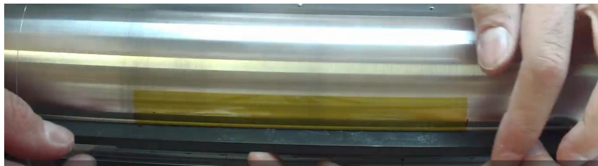
C. Glue under the lateral longeron, placed over the tape, insertion into the slots on the half-rings. + alignment tool during curing
