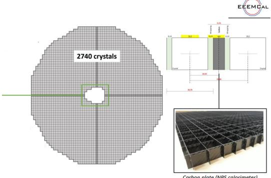
Carbon plate (NPS calorimeter)
