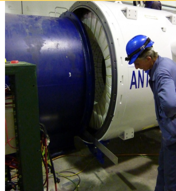
First trial mounting of one LAV module between two sections of the blue tube
