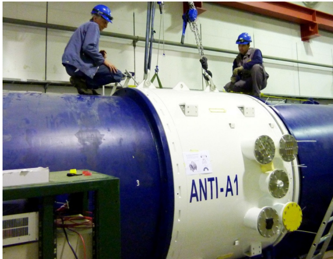
First trial mounting of one LAV module between two sections of the blue tube
