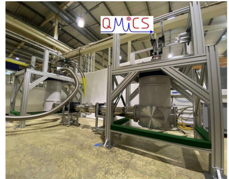
Eu Quantum Flagship Project led by WMI with Ziad Melhem Coordinating Oxford Instruments development of the CryoLink in QMiCS (Oct 2018-Jan 2021)
