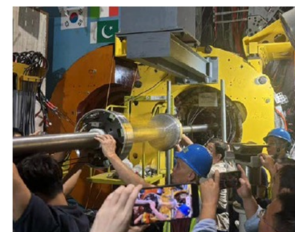
Pull out iMDC and and slide it out of the rail
