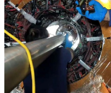
Push CF cylinder into place
