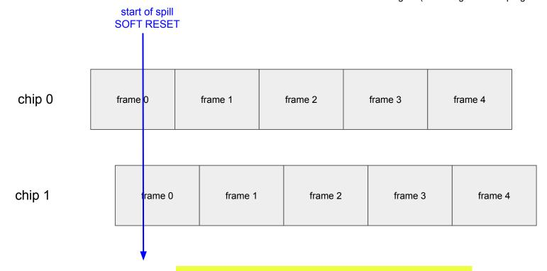
1. SOFT RESET does not align frames: misalignment not only on Frame counters but also on Frames
