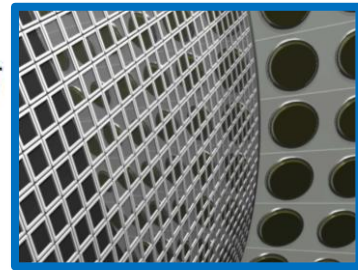
SiPMs on the \gamma entrance face + PMTs on the other faces
