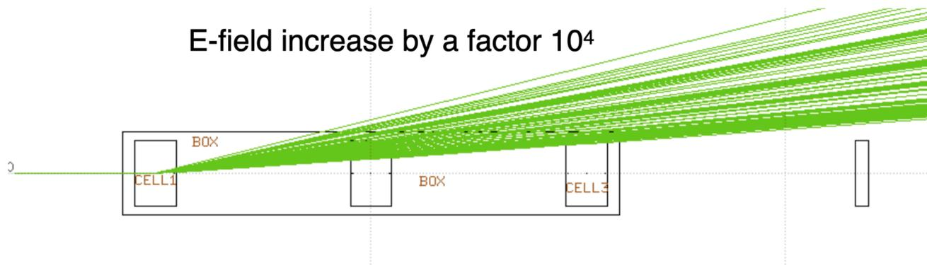
Deflection is a function of "impact parameter" of the incoming particle with respect to the sense wire
