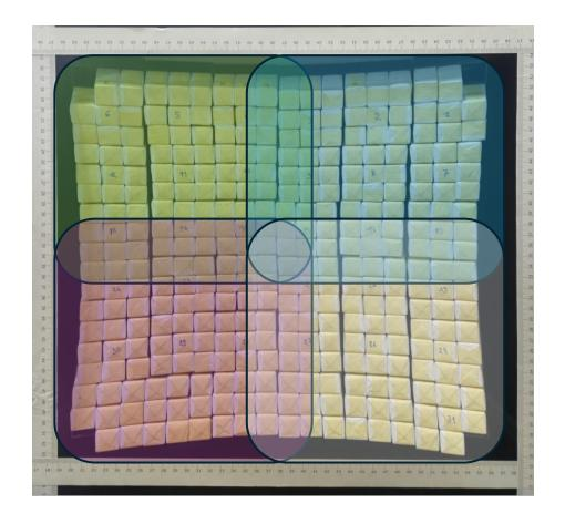
Calibration performed separately in four quadrants, about 4 hours per quadrant, at least 3 carbon energies and few proton energies.
