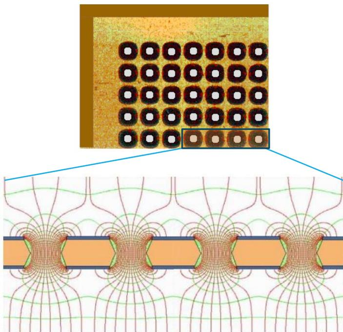
When a voltage is applied to the GEM foil an electric field develops within the holes. The electric field can be high enough ( $\sim 80 \text{ kV/cm}$ ) to make the **avalanche multiplication** develop.
