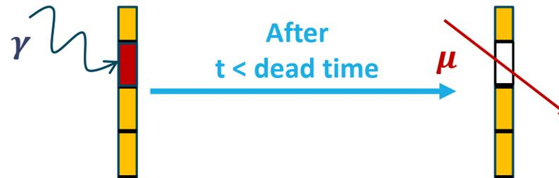
The drop of the efficiency for muons can be used to measure the **dead time** of the system.
