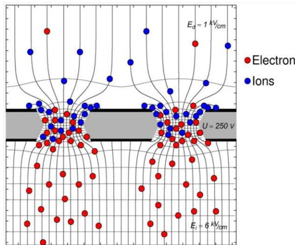
To enhance stability, GEM foils are often put in cascade. A typical configuration is that of three GEM foils: **Triple-GEM detectors**
