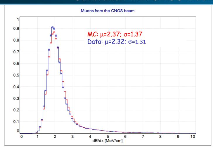
dE/dx distribution for real and MC muon tracks from CNGS events
