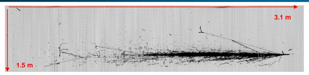
A  $v_e$ CC candidate from 2010 run. This event has 45 GeV energy with a single powerful 37 GeV e.m. shower at vertex with a longitudinal profile peaking at the expected position (~88 cm).
